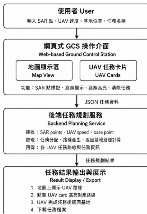
Figure 1: The architecture of the system
